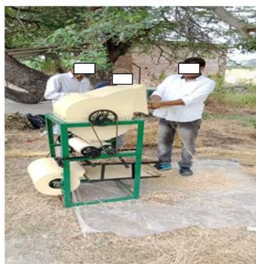
Fig. 2. Threshing of linseed crop by thresher
