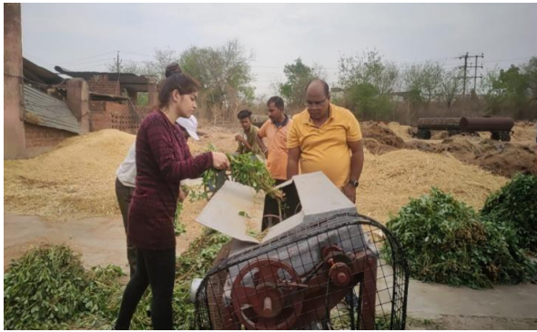
Fig. 9. Preliminary test of groundnut pod stripper
