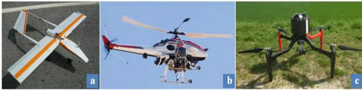
Fig. 4. Three examples of UAVs: a fixed-wing; b helicopter; c quadrotor (after Valavanis et al. 45)
