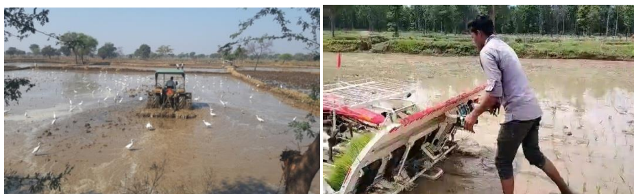
Fig.1. Puddling operation followed by mechanical transplanting of paddy
