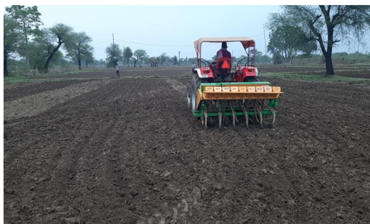
Fig.2. Direct seeding of rice using a seed cum fertilizer drill
