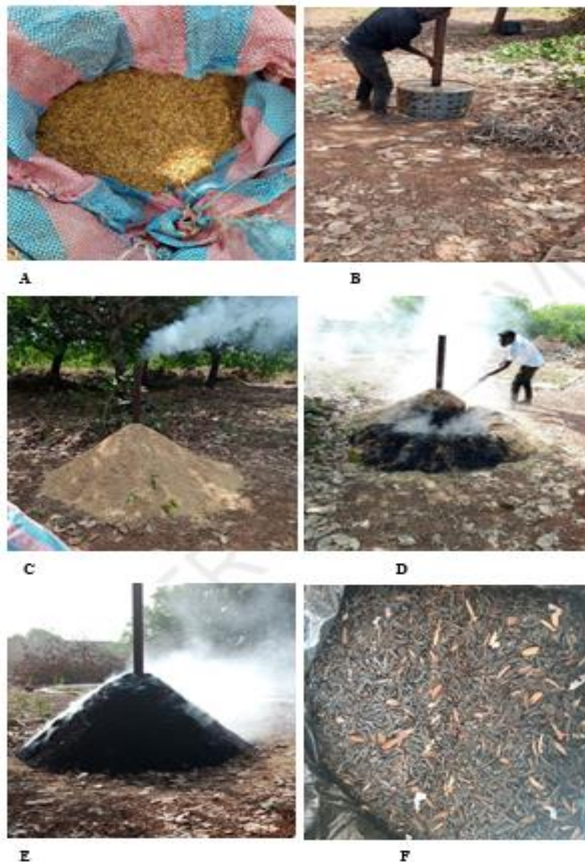
Fig. 3. Biochar production process
