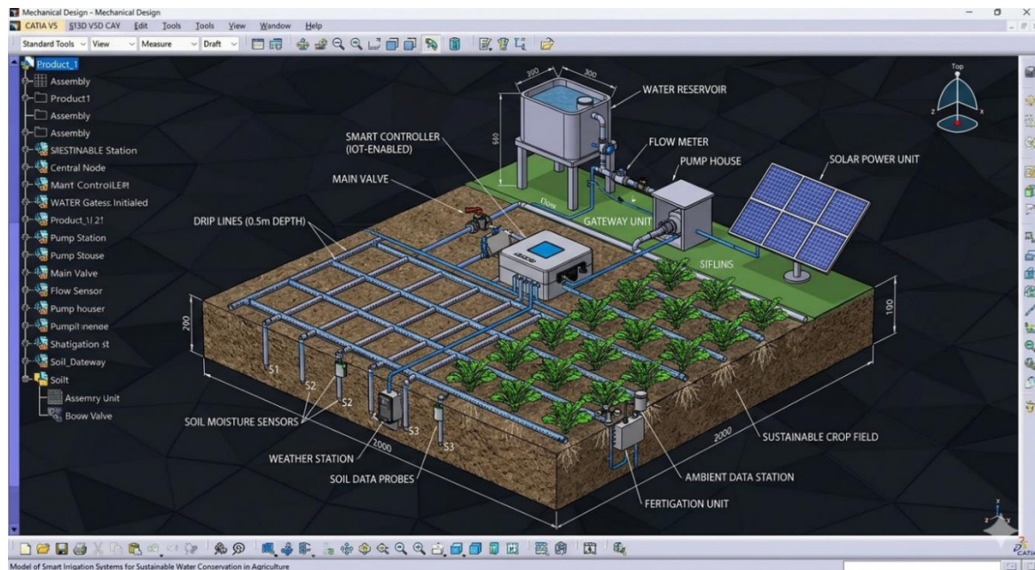
Fig. 1. CATIA model illustrates a comprehensive Smart Irrigation System designed for high-efficiency water management
