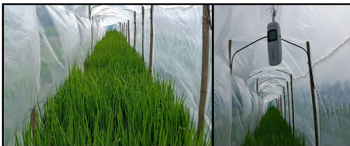
Fig. 1. Inner view of heat stress experimental unit consisting of automatic temperature recorder (Data logger)
